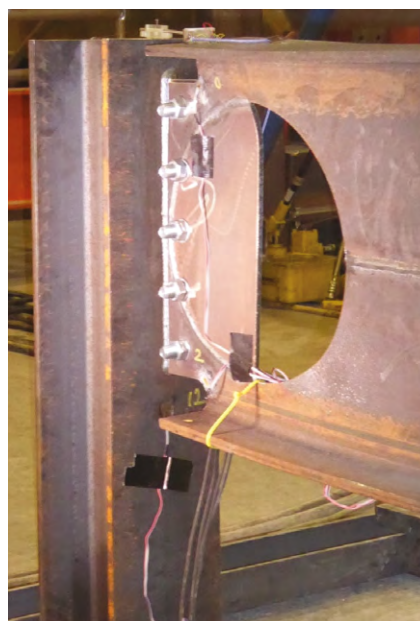
Figure 4 - Buckling of the half infill plate due to the transfer of shear from the top Tee
