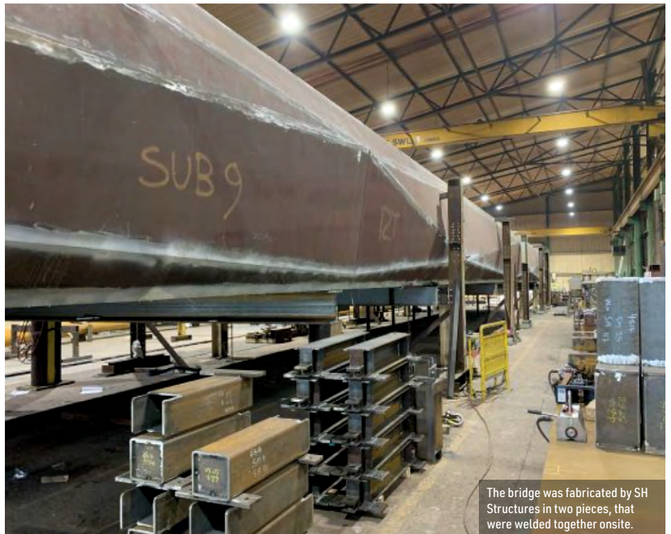
"Weathering steel was used in the design as the material develops a warm orange-brown industrial feel, which will help the bridge blend with the many nearby redbrick buildings."
