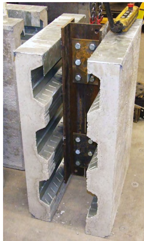
Figure 2a: Push out test specimen
