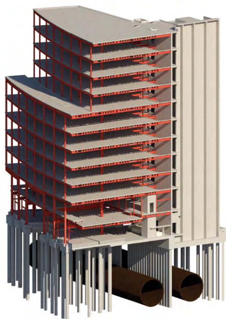
The structure straddles two Thameslink rail tunnels and so piles had to be installed between the tunnels and either side.
