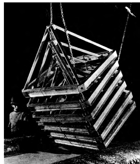
Stacked Unibat pyramids emerging from the galvanizing bath
